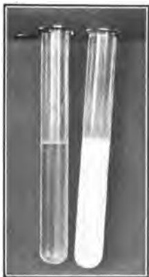
The limewater test. The tube at the right shows the effect of the carbon dioxide.
